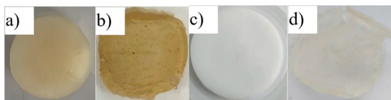
Figure 1. Appearances of CTS/PVA (2-3) and PVA hydrogel: a,c) gel as-prepared, and b,d) gel after drying
