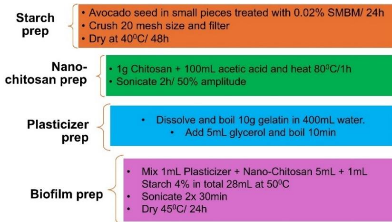
Figure 1. The combination between nano-chitosan and avocado seed derived-starch in biofilm production. (Adopted from Suhartini et al. )
