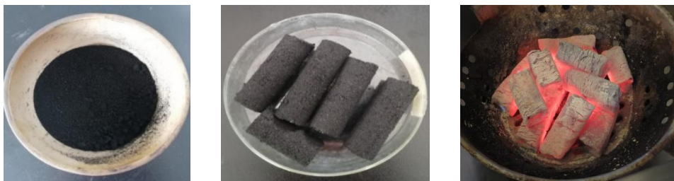
Figure 6. The solid fuel pellets are made from biochar, sugarcane bagasse, and coffee grounds
