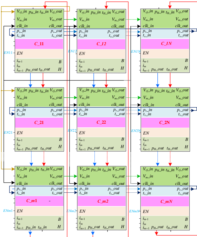
Figure 3. Decentralized control connection between cells with carrier phase angle interpolation algorithm for 2D structure
