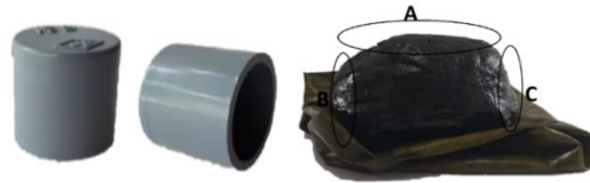
Figure 2. The illustration of the mold containing the sample and the cake in the order of sampling A, B, C (A is the middle of the crust, B and C is the edge of the crust)
